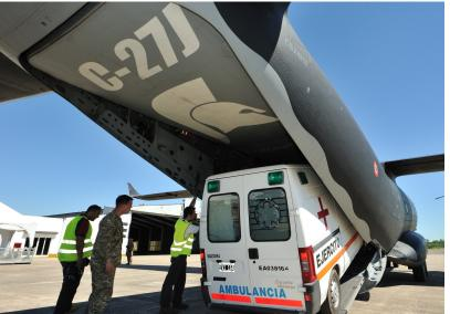
Wide cargo bay and outstanding floor strength for transport of heavy vehicles and full weight/height 88" x 108" standard pallets.
